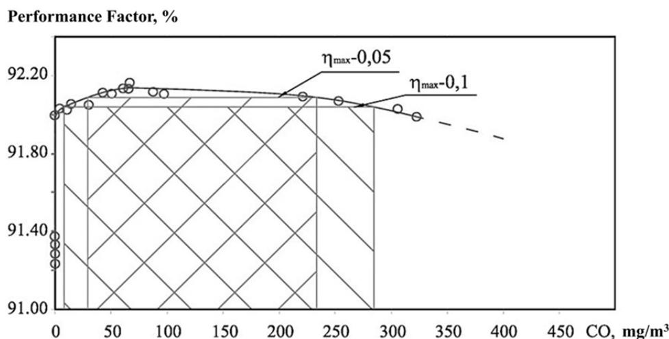
**Figure 4.** The range of CO concentrations in stack gases for optimal boiler performance: boiler E-75-3.9, natural gas combustion,  $D=75$  t/hr .
