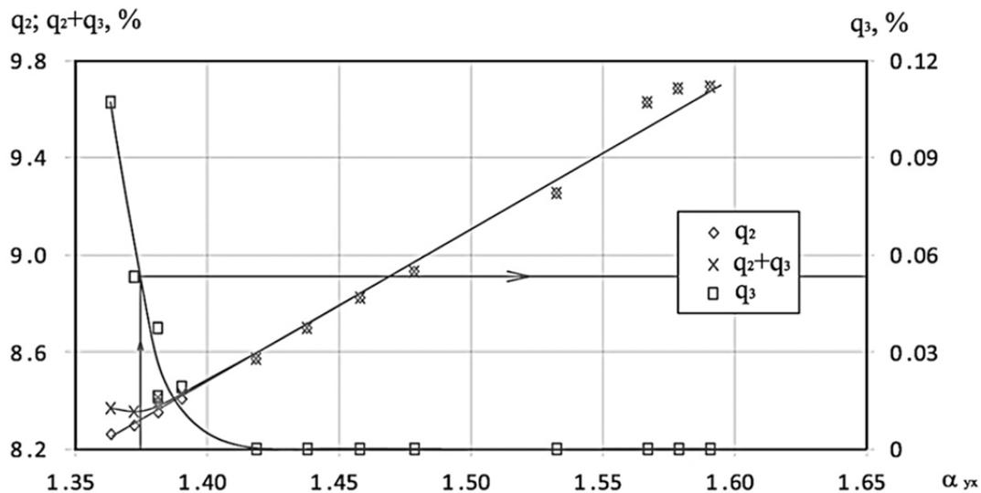
**Figure 3.** Excess air factor dependence of exhaust-gas-loss- $q_2$  and chemical incomplete combustion-loss- $q_3$  for boiler E-75-3.9 in the case of fuel oil combustion,  $D = 76-77$  t/hr.
