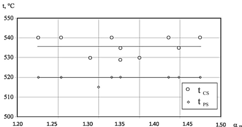
**Figure 5.** Dependence of platen superheater and convection superheater tube temperatures from excess air factor in stack gases: boiler E-500-13.8-560, natural gas combustion,  $D=370 - 410$  t/hr .
