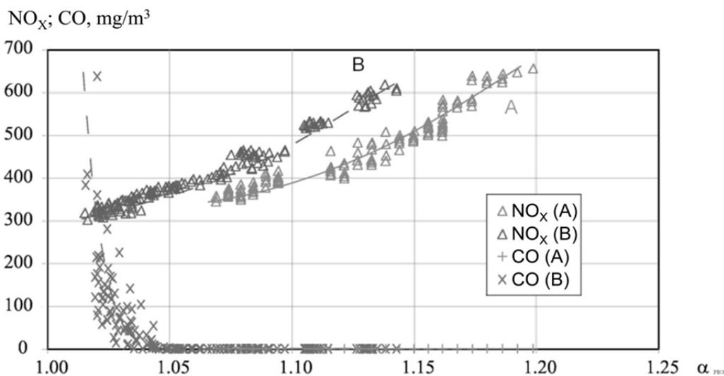
**Figure 6.** Concentrations of  $NO_x$  and CO, boiler E-480-13.8-560 (TGM-96), natural gas combustion,  $D=485$  t/hr : A – left side; B – right side.
